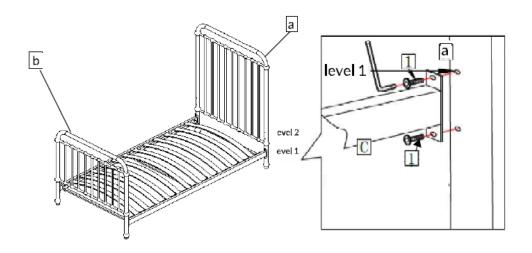
3. Attach the across bars (part d) to the siderails (part c) using the large bolts (part 2) and the hex nut (part 3) with the large allen key (part 5) and spanner (part 6) provided
